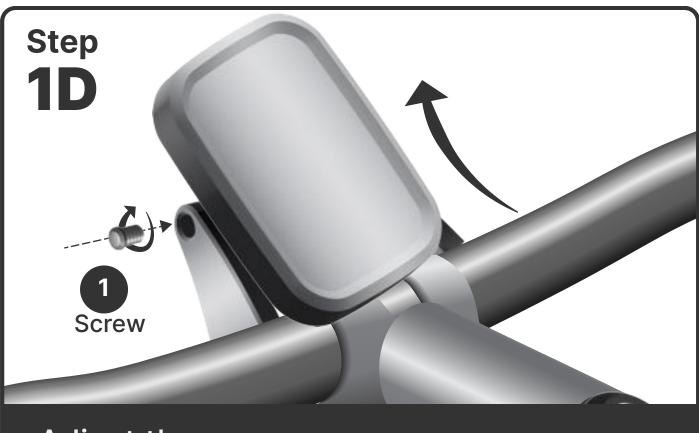
Adjust the screen Adjust the display position to fit your comfortable riding posture
