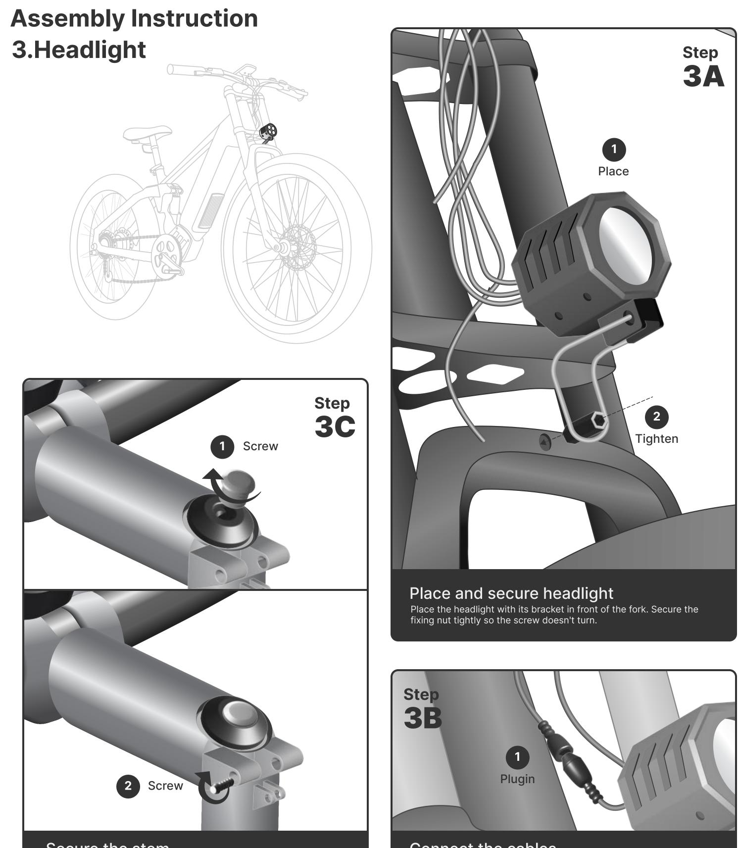
Secure the stem Tighten the screws on the stem end and on top of the stem
